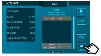
Pressing the DATA button provides a summary list of all test results for that GROUP. The specimen orientation is shown along with the details entered during the GROUP setup. This screen also allows you to select and delete individual test results.
