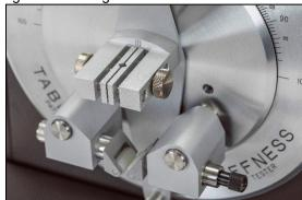
2. When required, mount the appropriate range weight to the bottom stud of the pendulum.
