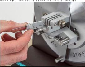
4. Loosen the knurled thumbscrew and slide it to the right. This will allow space for the specimen to be inserted between the pins.
