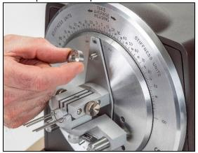
Place the specimen so it is above the second and fourth pins from the left and its back edge is parallel and about 1.5 mm from the pin holders.
