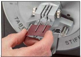
Slide the thumbscrew to the left until the two upper pins contact the test specimen. The upper pins should contact the test material, but not exert pressure on the test specimen such that they cause the pendulum to be deflected.
