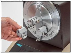
2. Place the *driving pin holder* on the two studs on the driving disc.
