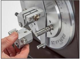
2. Mount the 10 Unit Compensator Range Weight to the top stud of the pendulum.
