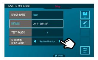
△ WARNING: When changing specimen material or testing direction (e.g. cross or machine direction), you must start a new group. Failure to do so will result in the data being recorded in the wrong group.
