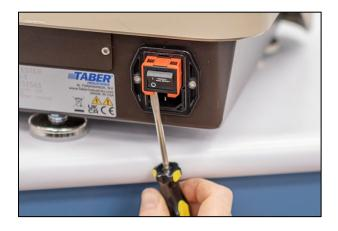
WARNING: Before replacing fuses, ensure the power switch is toggled to the OFF position.
