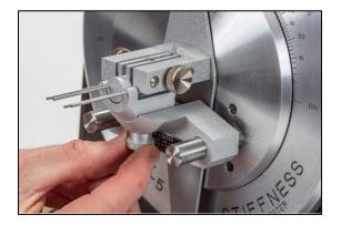
5. Mount the 10 Unit Compensator Range Weight to the top stud of the pendulum.
