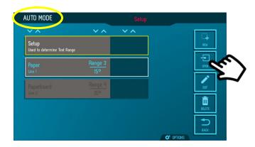
NOTE: Groups that are in different test ranges will not be selectable until the test range is changed.
