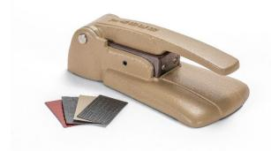
Specimens should be prepared both with the length parallel to the machine direction and with the length parallel to the cross-direction. At the very edge of each test specimen, mark or in some other way identify the machine or cross direction, being careful not to damage the specimens. DO NOT affix a label with adhesive or tape.
