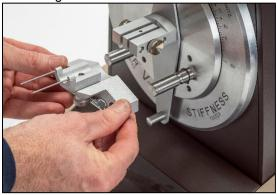
3. Open the jaws of the clamp fully by turning the clamp screws. Place the driven pin holder between the jaws of the clamp so "TOP" is facing upward and the positioning pins are in contact with the bottom surface of the clamp jaws. Tighten the clamp screws, ensuring the driven pin holder is centered in the clamp.
