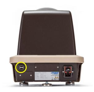
Once the USB drive is inserted, the operator will have the option to export all or just export the selected data grouping. A "CSV" file is sent to the USB drive which will allow the operator to transfer the data to a computer. Once this occurs, the CSV file can be opened by most spreadsheet applications.
